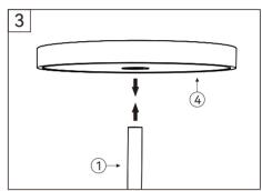
Insert the lamp head into one end of lamp pole
