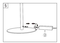
Plug the male end of the power output cable into the light pole input cable, rotate it  $90^{\circ}$  and fasten it.
