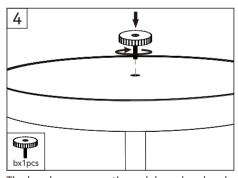
The hand screw goes through lamp head and rotates clockwise to secure it to the lamp pole
