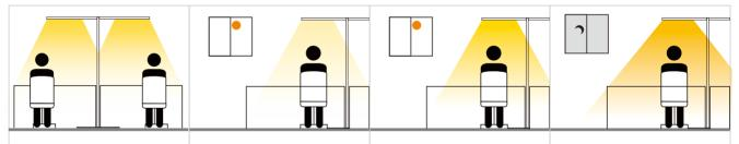
1. Turn on the light and dimming to a comfortable brightness, the daylight sensor will memory this lux value which performance on desk as a standard lux.
