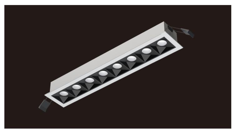
With extremely simple design and excellent craftwork, exquisite appearance looks with rich of texture. Collocated with micro reflector and anti-glare cover, it can realize55°beam angle and perfect light cutoff. UGR value is as low as 18. lamp is easy for installation and maintenance. Main material includes aluminum profile and PC. Typical value of light efficiency is 130lm/w, and lighting is of flicker free. Lamp supports 1-10V and DALI dimming.
