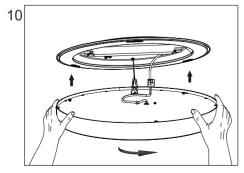
Align the three screw caps on the lamp body with the holes on the ceiling box and rotate them clockwise (about 10°) until they can no longer rotate.
