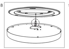
Attach the safety rope to the wire rope of the lamp body
