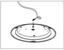
Thread the wires through the hole in the middle of the ceiling box.
