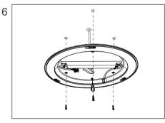
Secure the ceiling box to the ceiling with 4mm diameter screws.
