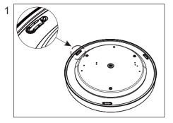
Rotate the ceiling box counterclockwise and remove it from the lamp body
