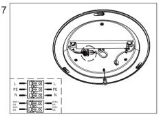
Connect the cable (make sure the power is off, AC200-240V).
