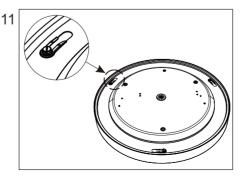
If the lamp body becomes slightly loose when pushed upward, it means it has been rotated in place.
