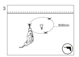
Drill three matching holes evenly in a 280mm diameter circle on the ceiling according to the size of the expansion screw plugs used.
