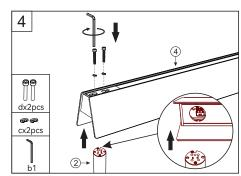
Insert the lamp head into one end of lamp pole Fix the lamp holder with screws
