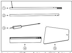
Product list: ① Down light pole ② Up light pole ③ Power supply ⑤ base plate ④ lamp body
