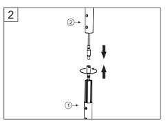
Plug the male end of the power output cable into the light pole input cable, rotate it  $90^{\circ}$  and fasten it.
