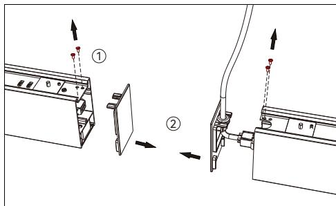
Loosen screw 1 as shown in the figure and remove the end cover on the side to be connected
