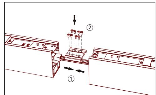
Secure the cascade block to the lamp body with screws.
